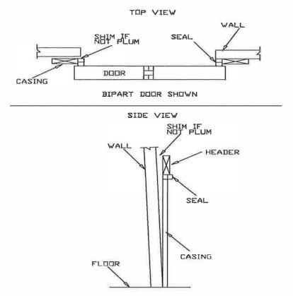
Plumb casing as shown and attach securely to wall using fasteners through holes pre-drilled
