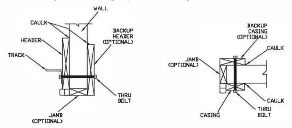
Use sealant to provide vapor seal between header, casings and wall. Compliance with above is essential to assure proper contact between door and gaskets. Seal and attach securely
