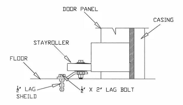
NOTE: Do not install stay roller to tightly against door panel. The door should open with very little effort when installed correctly. A slot is provided in the stay roller bracket to allow for some adjustment.
