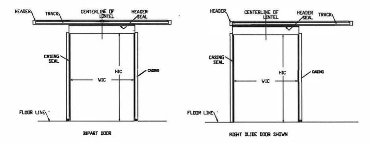
NOTE: If back-up header and casings or jamb covers are required, install as illustrated below.
