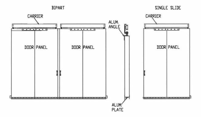
Once the securing angles and plates are attached to the door sections the door(s) is now ready to be attached to the door carrier. The door carriers simply bolt to the top of the door panel(s). Locate the threaded holes in the top of the door panel(s) and thread the adjustment nut into the threaded holes.
