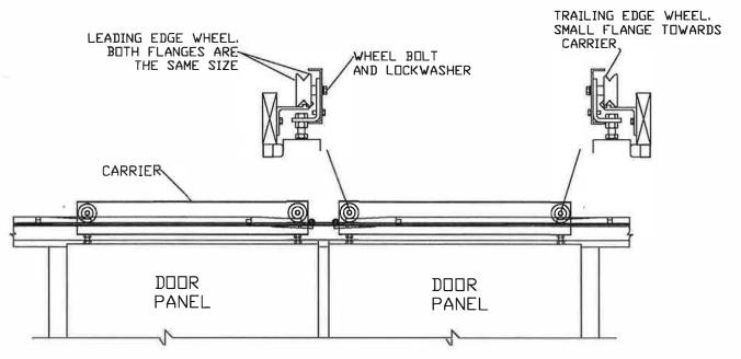
Once the door(s) are hung slide the door(s) back and forth to the open and closed positions to ensure that there are free from obstructions and there and there are no obstructions.
