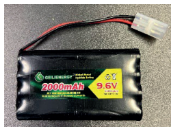
Battery (Factory installed in TFT enclosure)
