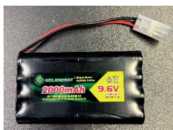
Battery (Factory installed in TFT enclosure)
