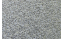
55% Al-Zn Alloy Coated Steel with Acrylic Coating (97)
